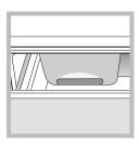
**MULTI-USE** box: fixed at the top of the compartment, this was designed to keep various foods for longer periods of time (for example eggs, butter or food in small containers); it prevents food odours from permeating into the refrigerator.
